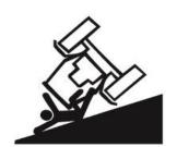
Take extreme care when operating the tank on sloping ground. Exercise extreme caution when turning on sloping ground. Especially with a partially filled tanker as the inertia will cause the weight of the tank to be thrown to one side of the tank.
